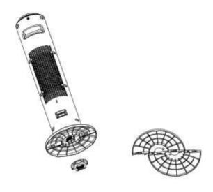
To fit the base to the body of the heater. Align the 4 clips on both sides of the base. Push together until both sides sit flush. Place on the bottom of the heater and secure using the plastic bolt provided.
